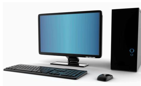
**System Unit:** is the most important part of a computer. It is like the brain. It does all the tasks that we want the computer to do. It also controls all the other parts, like the Monitor, Keyboard, and Mouse. These parts must be connected to the System Unit to work. In the system Unit the most important components, such as the Motherboard, CPU, Hard Drive, RAM, and Graphic Card (GPU) are stored.
