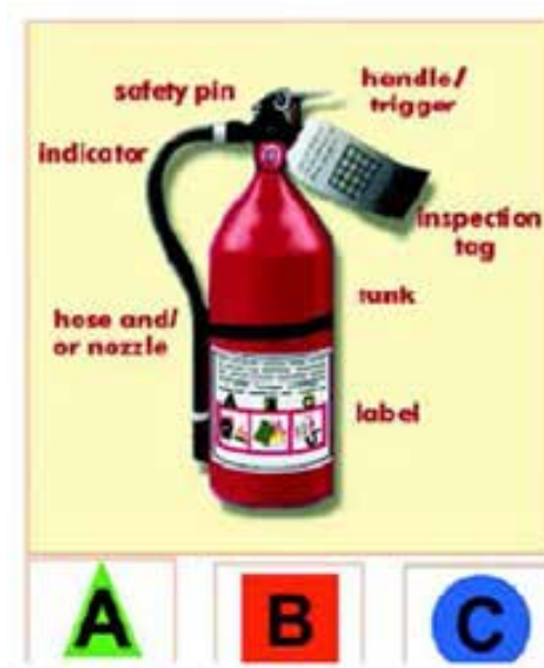
Figure 8. 1 Components of a fire extinguisher
