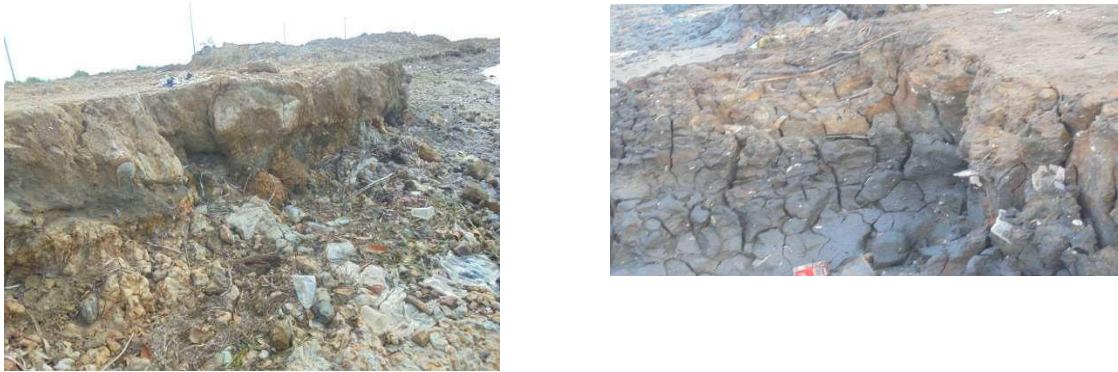
Plate 1: Soil composition made of clay and alluvial sediment at the proposed pier location
