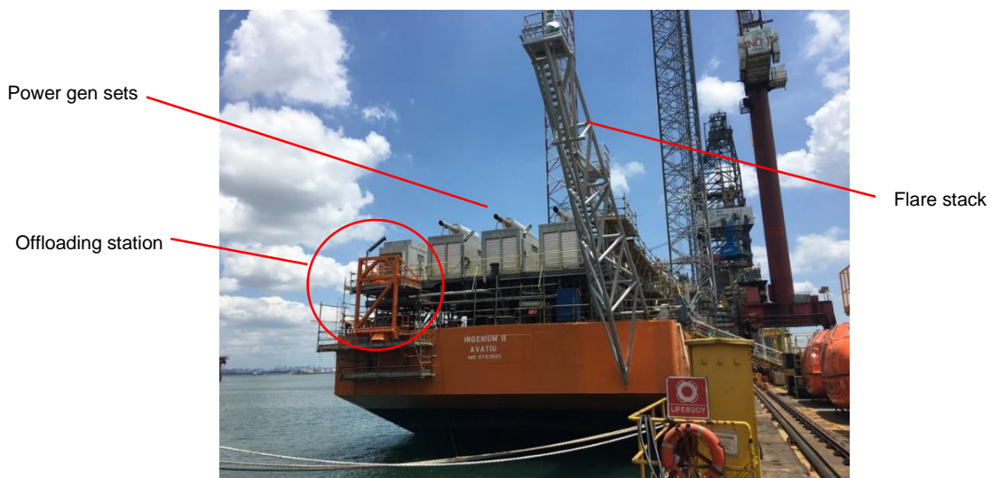
Stern of the Ingenium II showing flare stack, crude offloading station and power gen sets
