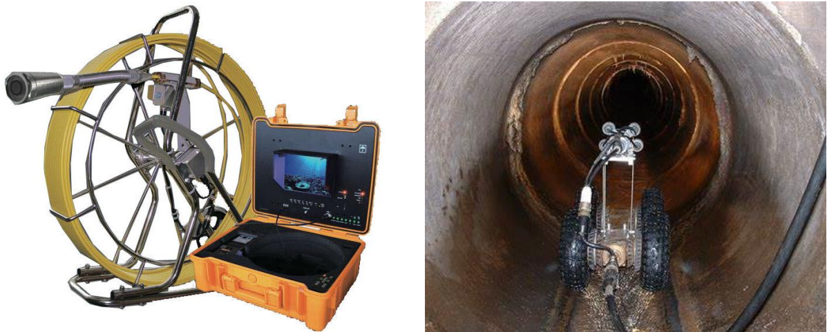
Figure 18. Portable TV system for small-diameter pipe (Source: EPA, 2003) and examination of lateral sewer by TV camera.
