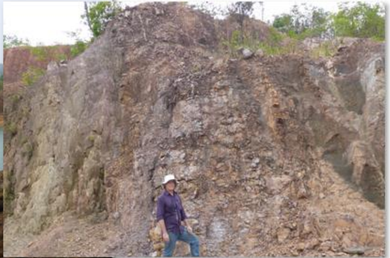
Khvav Open Pit Cu-Au mine. Altered porphyritic andesite hosts high-grade Cu-Au vein stockwork.
