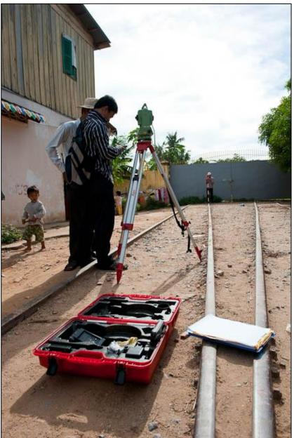
Figure 3. Working with a total station on the railway.
